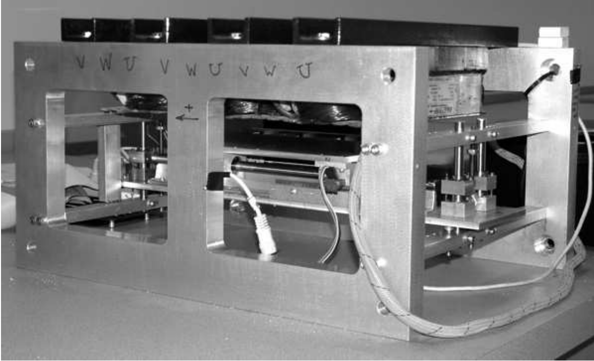
Figure 1: 2-DOF magnetic levitation hardware implementation
