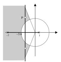
and choose a location for the two closed-loop system poles which is compatible with the region found in part (a) of the problem. For instance, we can choose closed-loop system poles at P = 3 + 4j (and its complex conjugate) as in the figure above. So, referring to (1), the problem is solved by setting  $\sqrt{16 - K} = 4j$ , or K = 32.
