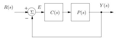
Prove that if the closed-loop transfer function  $\frac{Y(s)}{R(s)}$  has a pole-zero cancellation, then P(s)C(s) has a pole-zero cancellation.
