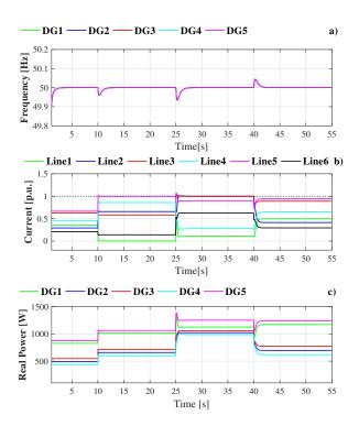
Fig. 5. Distributed congestion control response a) Frequency at each DG, b) Current in the lines, c) Real power injection for each DG
