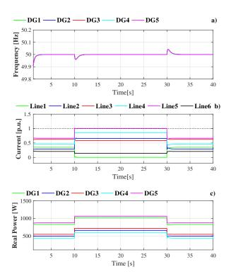
Fig. 10. Distributed congestion control response test by communication link failure between ( DG1 and DG2), and (DG3 and DG5) a) Frequency in each DG, b) Current from the lines, c) Real power injections for each DG
