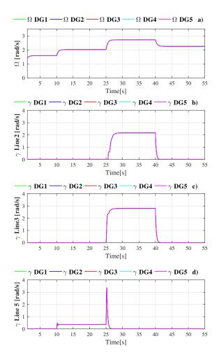
Fig. 6. a) Control action for frequency regulation, b) Congestion control action for line 2, c) Congestion control action for line 3, d) Congestion control action for line 5
