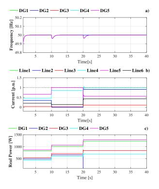
Fig. 8. Distributed congestion control response test by disconnecting DG2 a) Frequency in each DG, b) Current from the lines, c) Real power injections for each DG
