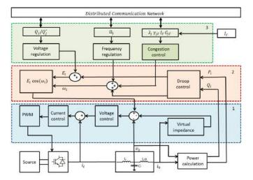
Fig. 1. Distributed control architecture for each DG
