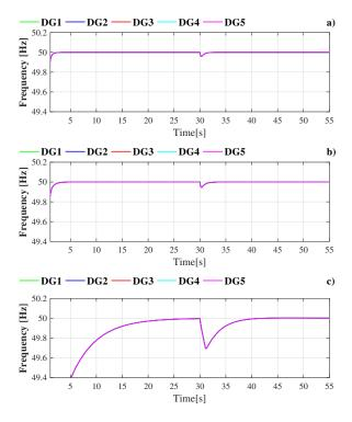
Fig. 11. Frequency response test with communication delay a) Without time-delay, b) With small time-delays  $\tau_i=0.05s$  , c) With large time-delays  $\tau_i=1s$
