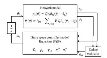
Fig. 3. Close-loop microgrid system.
