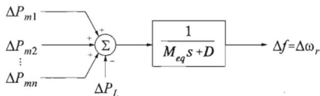
**Figure 11.16** System equivalent for LFC analysis
