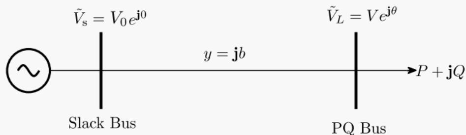
Active Power at PQ Bus:  $-P = V V_0 b \sin(\theta - 0)$
