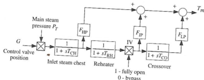
Figure 12.4 Block diagram of a reheat steam turbine.
