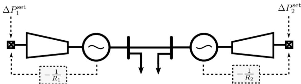
$$\Delta \mathbf{f}_{\text{ss}} = \frac{1}{\beta} \mathbf{1} \mathbf{1}^T \Delta \mathbf{P}_{\text{ss}}^{\text{set}} - \frac{1}{\beta} \mathbf{1} \mathbf{1}^T \Delta \mathbf{d}_{\text{ss}} \quad \text{so} \quad P(0) = \frac{1}{\beta} \mathbf{1} \mathbf{1}^T$$
