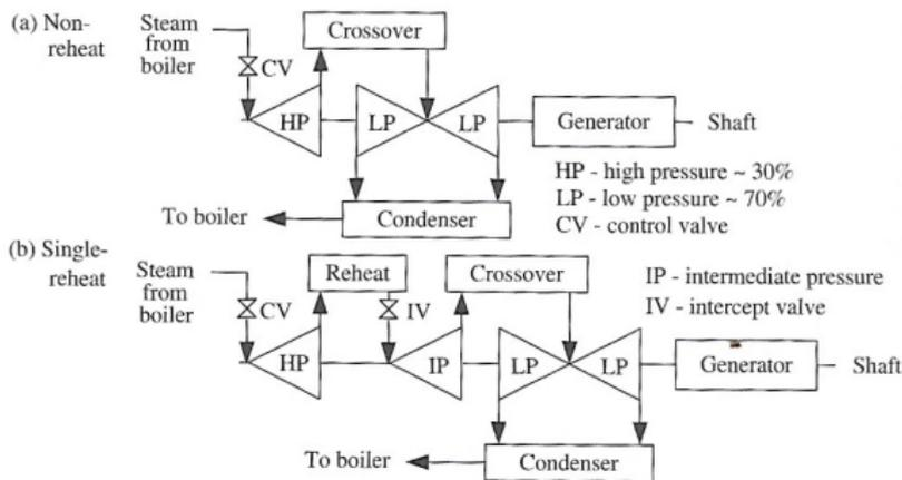
Figure 12.1 Steam turbine configurations: (a) a non-reheat unit and (b) a single-reheat unit.
