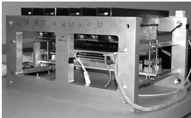
Fig. 1. 2-DOF magnetic levitation hardware implementation
