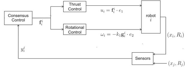
Fig. 1. Block diagram of the rendezvous control system for robot  $i$ .
