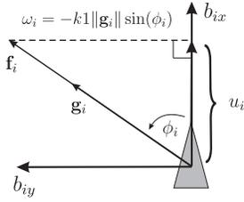
Fig. 2. Illustration of the control input  $u_i$  and reference angular speed  $\omega_i$  in (5).
