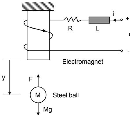
Figure 1: block diagram of a magnetic ball-suspension system
