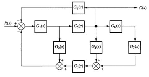
2. Reduce the following bock diagram to a single block, T(s) = C(s) / R(s).
