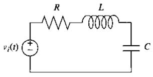
where  $C = 10 \,\mu\text{F}$ , find *R* and *L* to yield 15% overshoot with a settling time of 2 ms for the capacitor voltage. The input, v(t) is a unit step.
