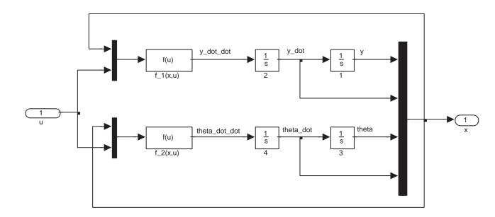
The Fcn blocks are used to specify the nonlinear functions in the system. Based on these suggestions, set up the complete SIMULINK model corresponding to the inverted pendulum on a cart system. Save your model in SIMULINK as, say, invertpen.slx.
