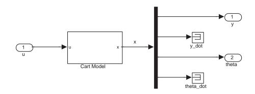
where the input u to the nonlinear state equation is a force input to the cart, and the outputs y and  $\theta$  are the position of the cart and the angle of the pendulum with respect to the vertical, respectively. ion. The block "Cart Model" corresponds to the nonlinear state equation and is a subsystem of the SIMULINK model. The cart model block can be built in the form described by the following figure:
