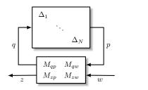
$$\begin{bmatrix} p_1 \\ \vdots \\ p_N \end{bmatrix} = \begin{bmatrix} \Delta_1(q_1) \\ \vdots \\ \Delta_N(q_N) \end{bmatrix}$$
