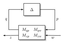
In a linear fractional representation (LFR) of uncertainty, an uncertain input-output system  $z=\mathcal{F}(M,\Delta)(w)$  is described using a feedback interconnection between (i) a causal LTI system M, and (ii) a causal system  $\Delta$ .
