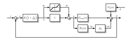
$$p = \left[ \begin{smallmatrix} p_1 \\ p_2 \end{smallmatrix} \right], \quad q = \left[ \begin{smallmatrix} q_1 \\ q_2 \end{smallmatrix} \right], \quad \Delta(q) = \left[ \begin{smallmatrix} \operatorname{deadzone}(q_1) \\ \Delta_2(q_2) \end{smallmatrix} \right]$$
