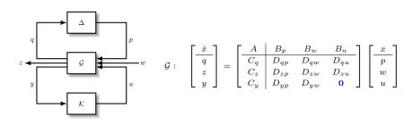
**Problem:** Design a (dynamic) feedback controller  $\mathcal K$  such that the closed-loop system achieves **robust performance** on the channel  $w\mapsto z$ .
