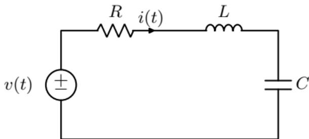
$$LC \frac{d^2 i(t)}{dt^2} + RC \frac{di(t)}{dt} + i(t) = C \frac{dv(t)}{dt}$$
