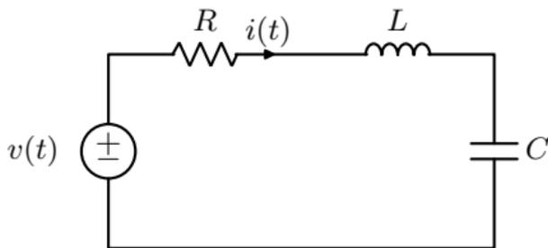
$$\begin{aligned} \frac{d^2 i(t)}{dt^2} + \frac{R}{L} \frac{di(t)}{dt} + \frac{1}{LC} i(t) \\ = \frac{1}{L} \frac{dv(t)}{dt} \end{aligned}$$
