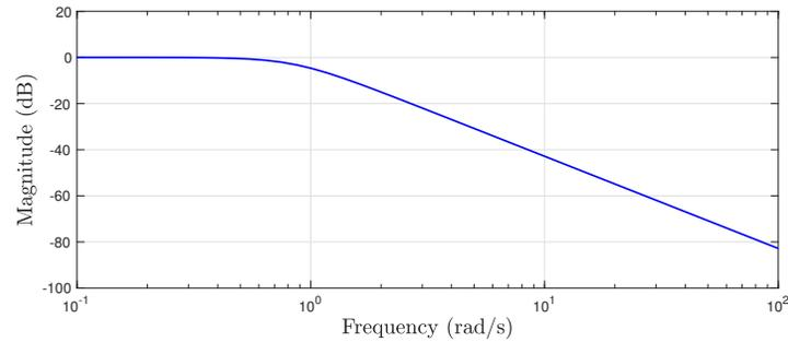
$$\begin{aligned} \omega_{\text{bw}} \approx 1.2 \text{ rad/s} &\implies \omega_s \geq 25(1.2) = 30 \text{ rad/s} \\ &\implies T \leq \frac{2\pi}{30} \approx 0.2 \text{ s} \end{aligned}$$
