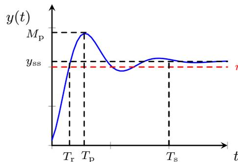
► **Final value theorem:** if  $f(s) = \mathcal{L}\{f(t)\}$  is rational and proper, with all poles of  $sf(s)$  contained in  $\mathbb{C}_-$  then  $f_{ss} = \lim_{t \rightarrow \infty} f(t)$  exists and
