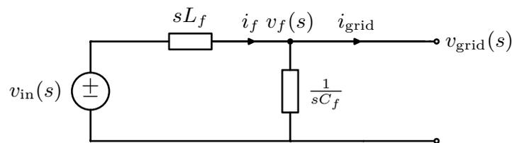
$$\text{inductor current: } i_f(s) = \frac{1}{sL_f}(v_{in}(s) - v_f(s))$$
