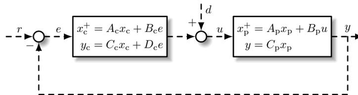
$$\begin{aligned} x_p^+ &= A_p x_p + B_p (d + y_c) & x_c^+ &= A_c x_c + B_c (r - y) \\ y &= C_p x_p & y_c &= C_c x_c + D_c (r - y) \end{aligned}$$
