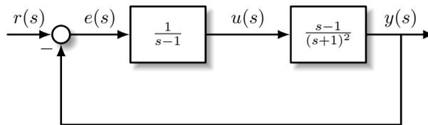
$$\begin{aligned} \Rightarrow \quad \Pi(s) &= (s+1)^2(s-1) + (s-1) \\ &= (s-1)(s^2 + 2s + 2) \end{aligned}$$
