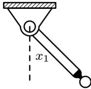
$$\begin{aligned} 0 &= \bar{x}_2 \\ 0 &= -\frac{g}{\ell} \sin \bar{x}_1 + \frac{1}{m\ell^2} \bar{u} \end{aligned}$$
