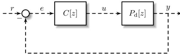
**Tracking problem:** Given a plant  $P_d[z]$ , design a controller  $C[z]$  such that the closed-loop system is feedback stable and
