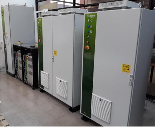
Fig. 5. Experimental System based on five Triphase power converters with nominal powers between 5kW to 30kW (each one). They are configured to emulate the topology of Fig. 6.
