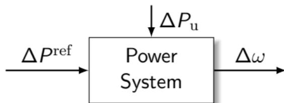
**Control inputs:** Power set-points to devices  $\Delta P_i^{\text{ref}}$
