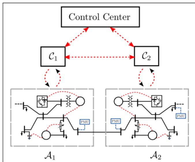
Bulk grid divided into small **local control areas**  $\mathcal{A}_1, \dots, \mathcal{A}_N$  (e.g., a few substations each)
