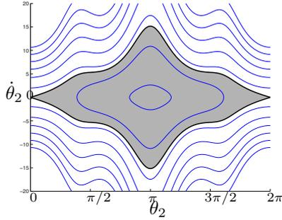
Fig. 4. Energy level sets for double pendulum on the virtual constraint  $\theta_1 = \sin(2\theta_2)/4$ .
