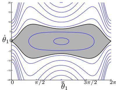
Fig. 5. Energy level sets for double pendulum on the virtual constraint  $\theta_2 = \theta_1 + 2 \arctan[\tan(-\theta_1/2)(1 + \sqrt{2})]$ .
