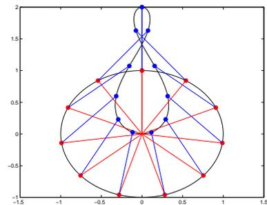
Fig. 3. Configurations of the double pendulum with the virtual constraint  $\theta_2 = \theta_1 + 2 \arctan[\tan(-\theta_1/2)(1 + \sqrt{2})]$ .
