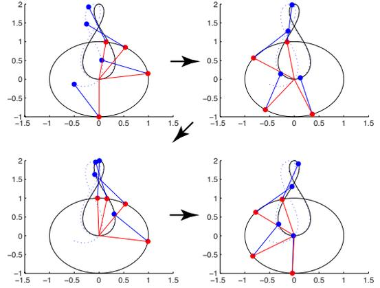
Fig. 6. Stabilization of the constraint  $\theta_2 = \theta_1 + 2 \arctan[\tan(-\theta_1/2)(1 + \sqrt{2})]$ .
