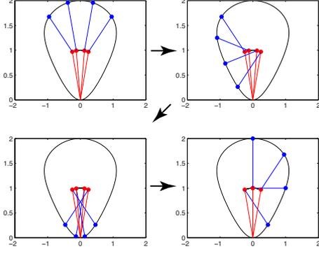
Fig. 2. Configurations of the double pendulum with the virtual constraint  $\theta_1 = \sin(2\theta_2)/4$ .
