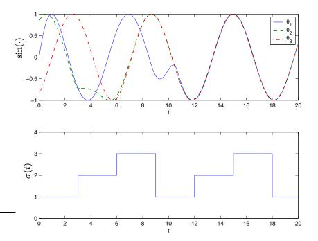
FIG. 3.4. Synchronization of three oscillators with a dynamic interaction structure.
