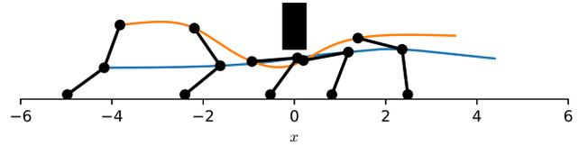
Fig. 5. Configuration of the cart-acrobot along a constraint satisfying the conditions of Problem 2
