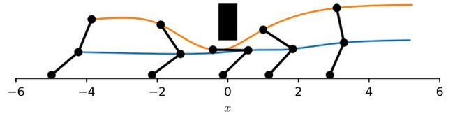
Fig. 4. Configuration of the cart-acrobot along a constraint satisfying the conditions of Problem 1
